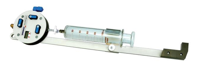
The sampling syringes (100 ml - fully made of glass) are gas-tight and equipped with a special valve. Together with a flexible PFT tube, the syringes can be directly connected to the oil-sampling flange of the transformer.
